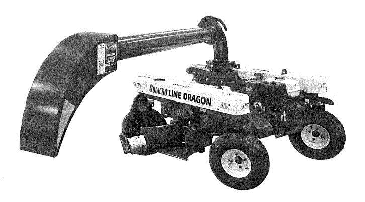
If you want to make using concrete pump hoses an even more efficient process, you need the Somero® Line Dragon® Line-Pulling and -Placing System. These remote-controlled hose-handlers are packed with powerful engines and load-sensing variable-displacement hydraulics that move lines with ease. Besides being the most nimble option on the market, these machines are sure to enhance productivity, create labor savings, and reduce the risk of injury that comes with moving pump hoses by hand.
